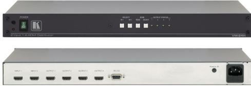
The VM-24H is a distribution amplifier for HDMI signals. The unit reclocks and equalizes one of two selectable input signals and distributes it to four identical outputs
